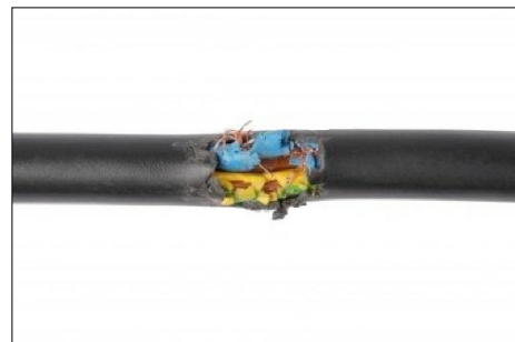
Damaged electric cable
